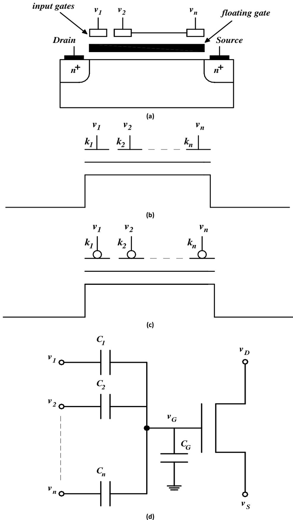
Fig. 3. a) Basic structure of an N-channel FGMOS transistor with the floating gate and the  $n$ -input control gates shown; b) the adopted symbol for the N-channel FGMOS transistor [66]; c) the adopted symbol for the P-channel FGMOS transistor [66]; d) the adopted equivalent circuit of the FGMOS transistor [67] ( $v_D$  and  $v_S$  are the drain and source voltages, respectively).
