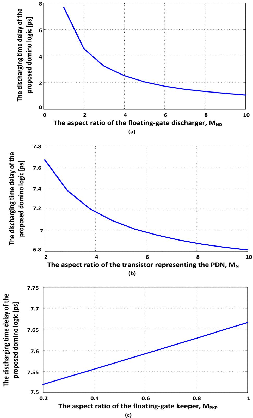
Fig. 7. Propagation delay of the proposed domino logic versus the: a) aspect ratio of the transistor,  $M_{ND}$ ; b) aspect ratio of the transistor representing the PDN; c) aspect ratio of the keeper transistor.
