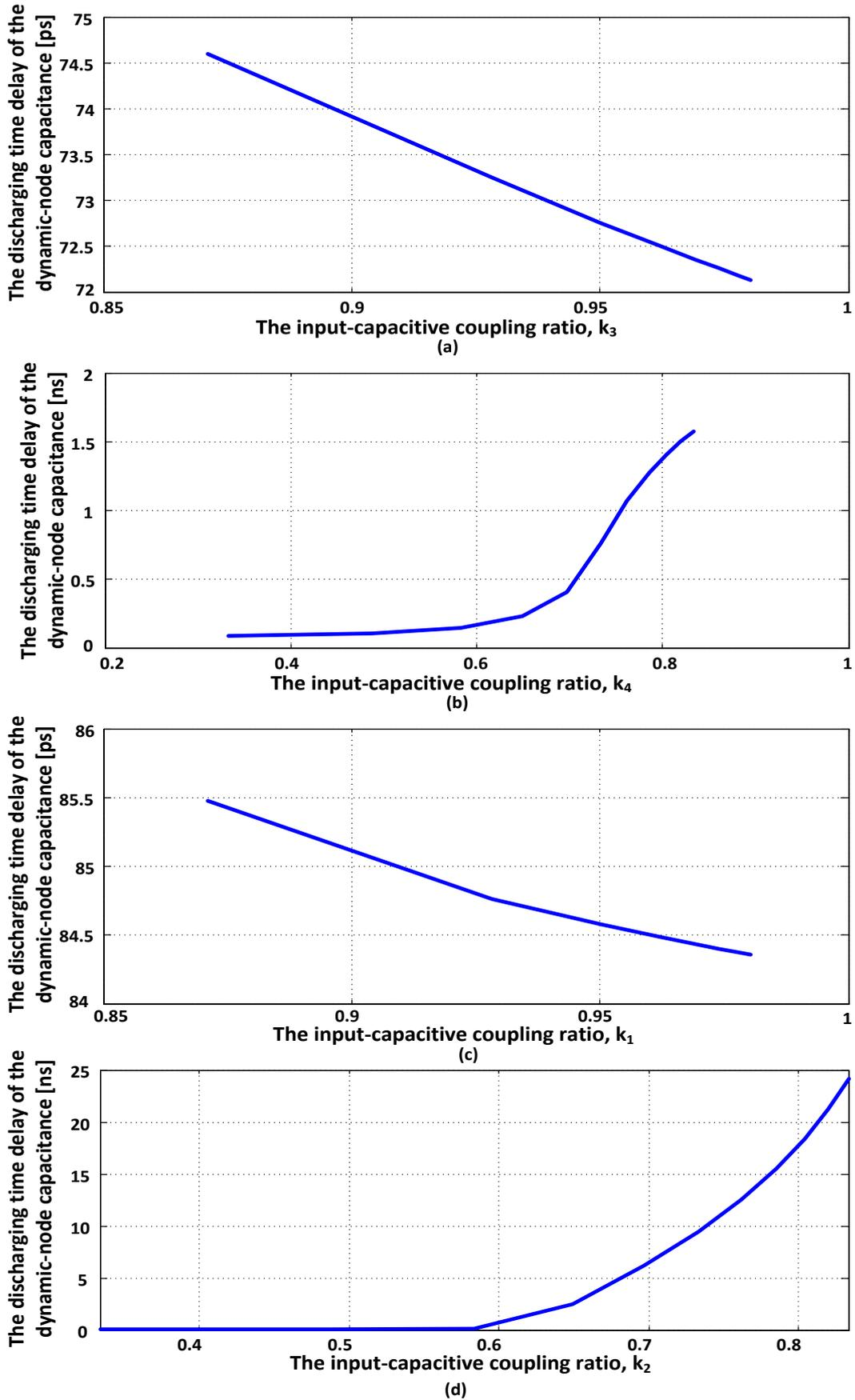
Fig. 11. Relationship between the discharging time delay of the dynamic-node capacitance and each of the following input-capacitive coupling ratios: a)  $k_3$ ; b)  $k_4$ ; c)  $k_1$ ; d)  $k_2$  for AND gates.
