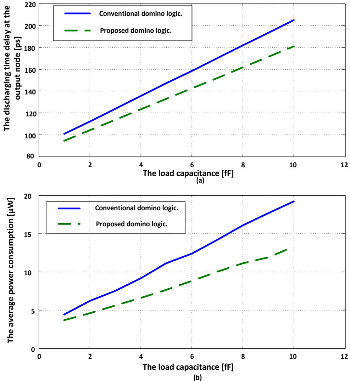
Fig. 12. Effect of the fan-out capacitance on the: a) discharging time delay; b) average power consumption.
