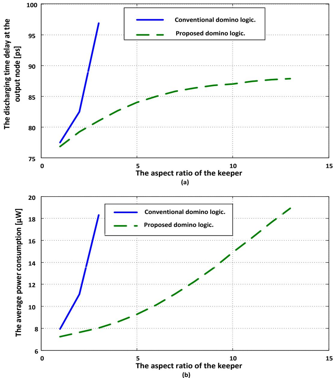
Fig. 15. Effect of the keeper size on the: a) discharging time delay; b) average power consumption.
