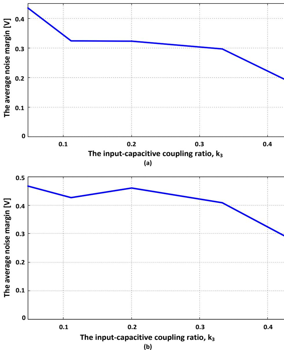
Fig. 9. Relationship between the input-capacitive coupling ratio,  $k_3$ , and the average noise margin for: a) one activated input; b) all activated inputs in case of parallelly connected devices.
