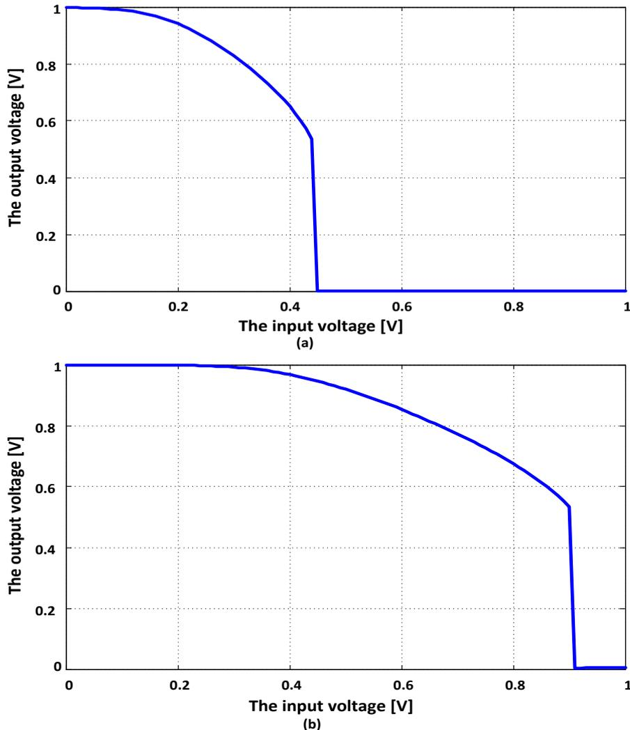
Fig. 8. Voltage-transfer characteristics of the conventional domino logic for the case of: a) parallelly connected devices with eight activated inputs; b) serially connected devices in the PDN.
