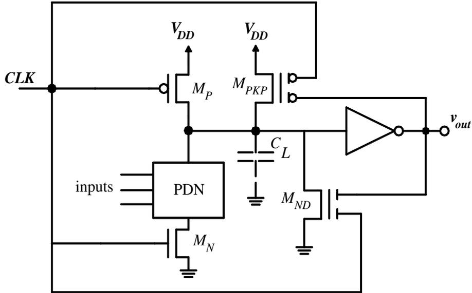
Fig. 4. Circuit schematic of the proposed domino logic ( $K$  and  $D$  in  $M_{PKP}$  and  $M_{ND}$  refer to keeper and discharger, respectively).
