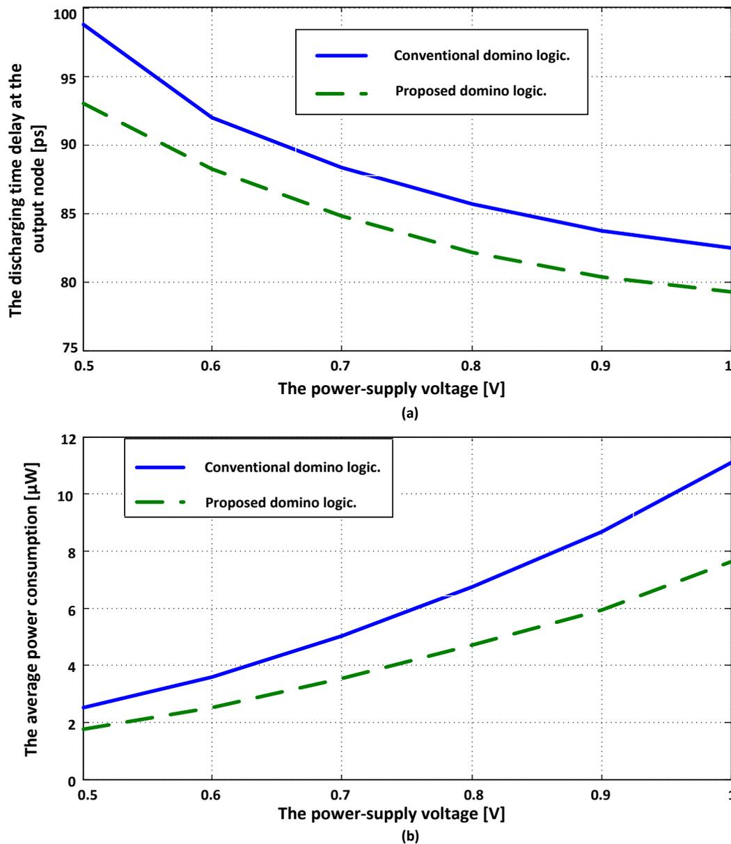
Fig. 13. Effect of the power-supply voltage on the: a) discharging time delay; b) average power consumption.
