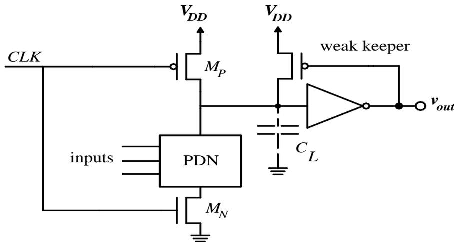
Fig. 1. Circuit schematic of the standard CMOS domino logic [13].
