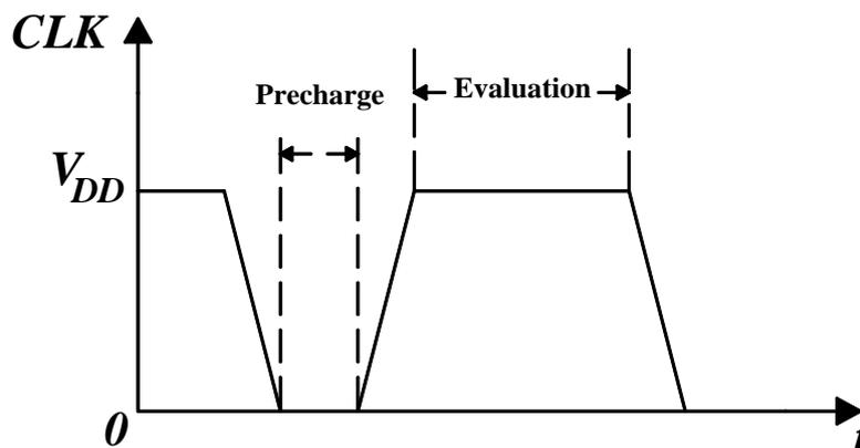
Fig. 2. The  $CLK$  signal as a function of time during the precharge and evaluation phases [13].
