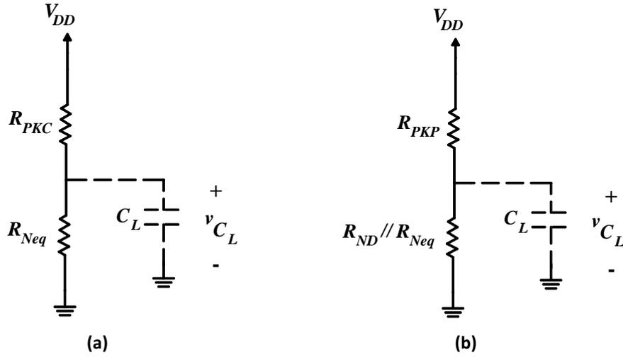
Fig. 6. Equivalent circuit of the: a) conventional; b) proposed domino logic (letters *N*, first *P*, second *P*, and *C* refer to NMOS, PMOS, proposed, and conventional, respectively).
