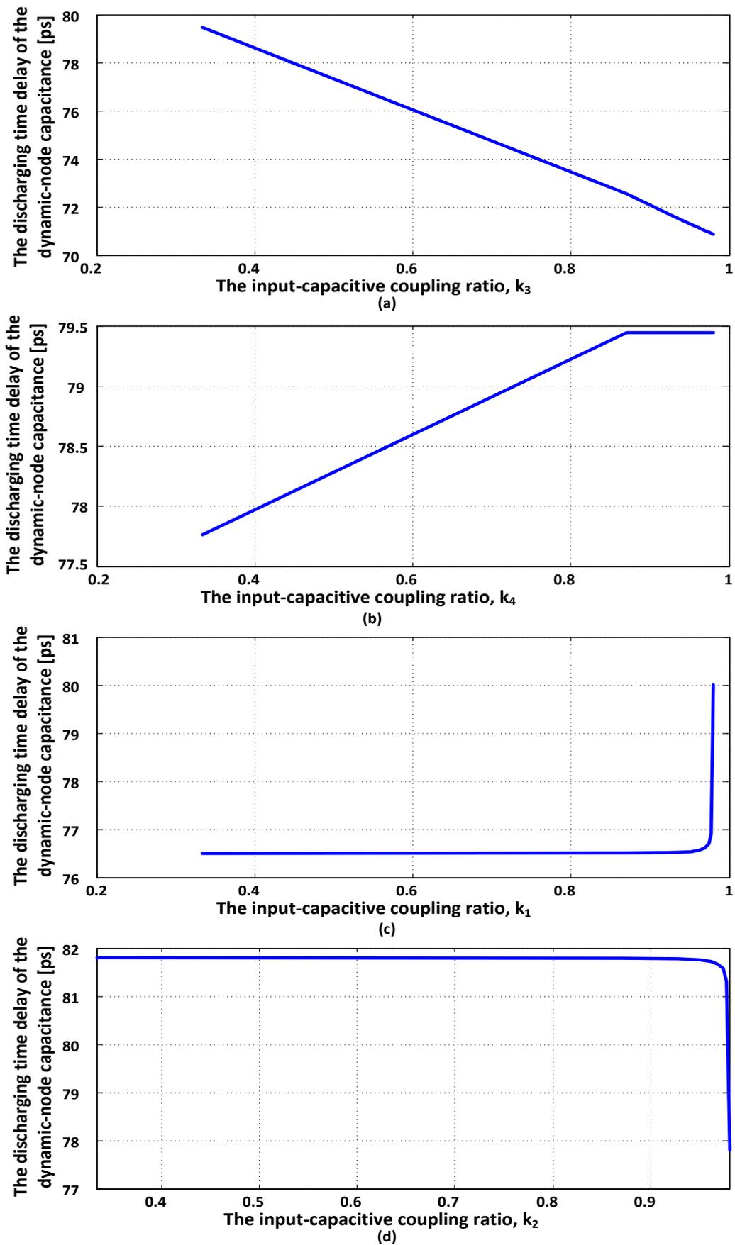
Fig. 10. Relationship between the discharging time delay of the dynamic-node capacitance and each of the following input-capacitive coupling ratios: a)  $k_3$ ; b)  $k_4$ ; c)  $k_1$ ; d)  $k_2$  for OR gates.
