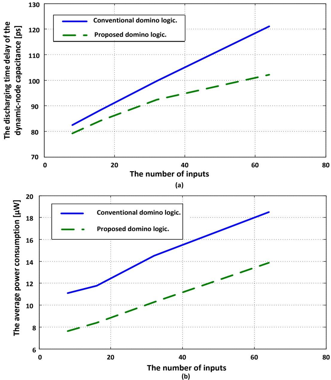
Fig. 14. Effect of the number of inputs on the: a) discharging time delay of the dynamic-node capacitance; b) average power consumption.
