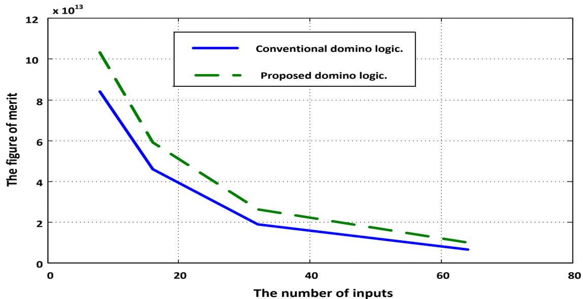
Fig. 16. The proposed figure of merit versus the number of inputs.
