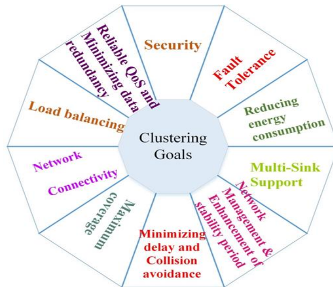
Fig. 1. The objectives of clustering procedures in WSN.
