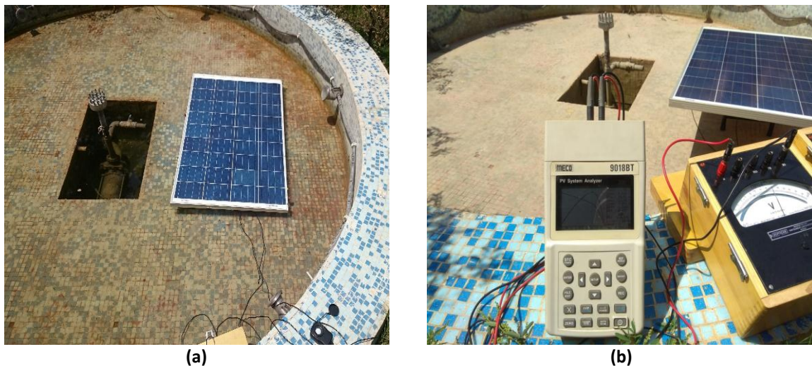
Fig. 2. Experimental setup: a) FSP system; b) LBP system.
