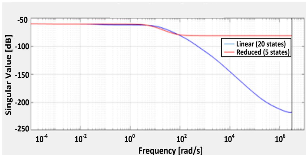
Fig. 6. Linear and reduced order model states.
