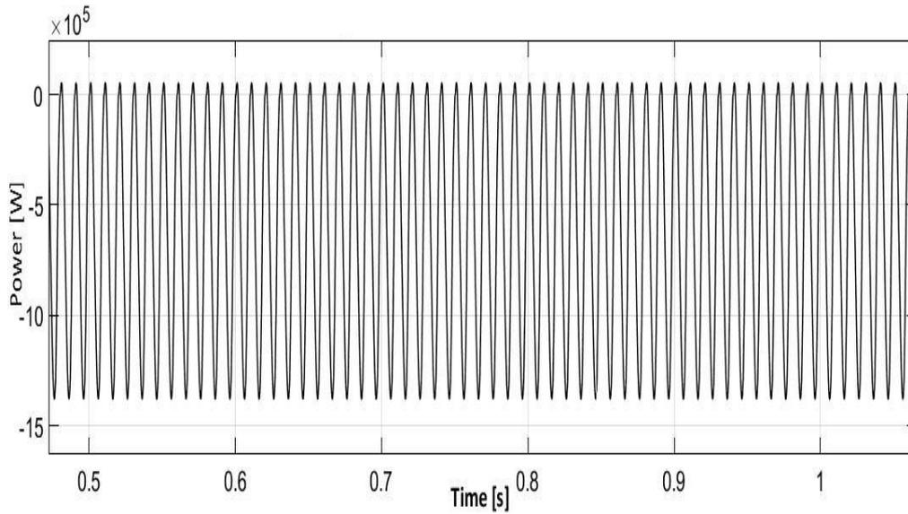
Fig. 12. Output power of the reduced order model.
