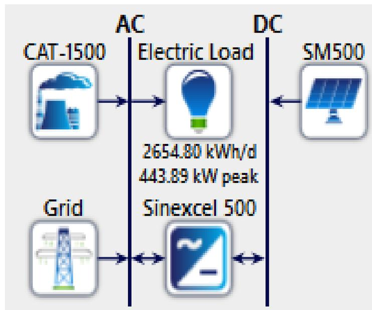
Fig. 3. Schematic diagram of the microgrid system.
