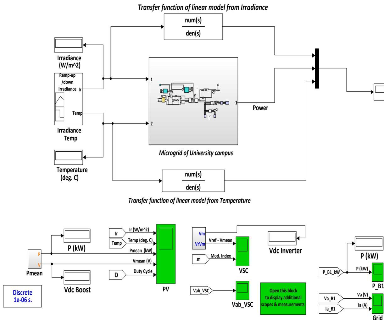
Fig. 5. Linearized microgrid model.
