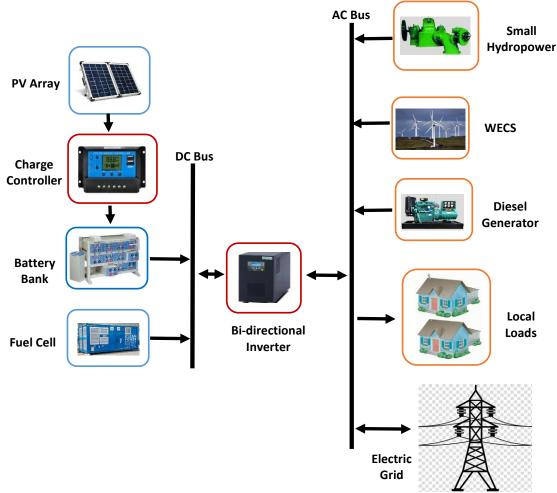
Fig. 1. Block diagram of a typical grid-connected HES.
