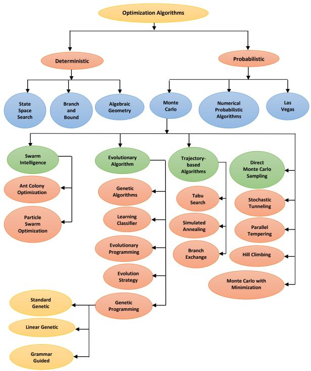
Fig. 2. Classification of optimization algorithms based on operating principles.
