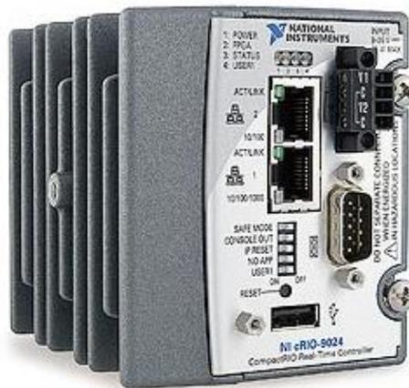
Fig. 11. The NI cRIO-9024 real-time controller.
