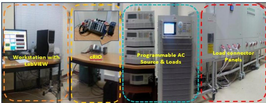
Fig. 2. The experimental setup in a power quality laboratory.
