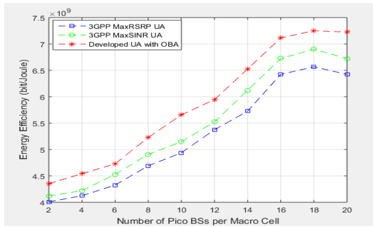
Fig. 3. Energy efficiency versus number of pico BSs per macro cell for user association algorithms
