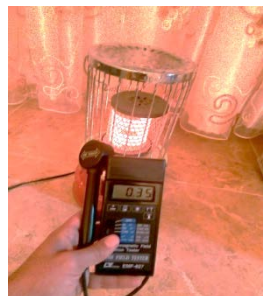
Fig. 5. Reading EMF for an electric heater
