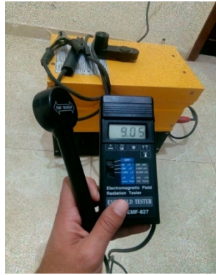
Fig. 6. Reading EMF for a welding machine
