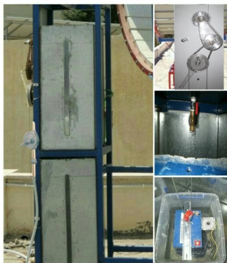
Fig. 2. Gear box unit with three types of pulley
