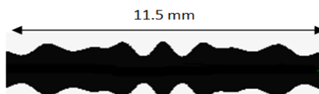
Fig. 10. Compacted quarter wave transformer
