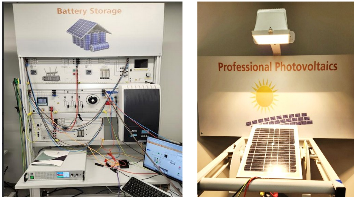
Fig. 10. complete solar setup: a) wiring connection hardware; b) solar panel altitude emulator.
