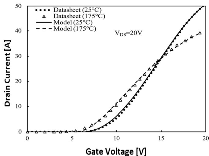
Fig. 5. Transfer characteristics of the proposed model and CoolSiC MOSFET IMZ120R140M1H from [24] at 25 °C and 175 °C.
