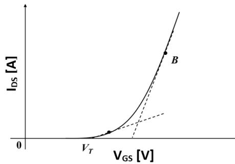
Fig. 2. Extraction procedure for starting point initial values of  $B$  and  $V_T$  parameters.
