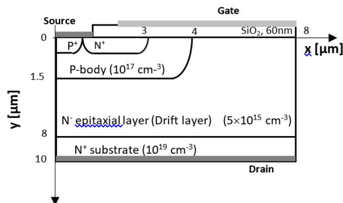
Fig. 1. Half-cell structure of the SiC MOSFET used in TCAD simulations.
