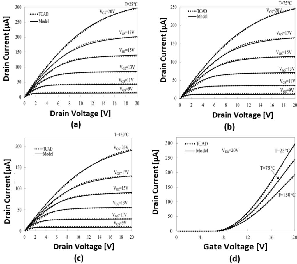
Fig. 6. Output characteristics of model and TCAD simulation at: a) 25 °C; b) 75°C; c) 150 °C and d) transfer characteristics.
