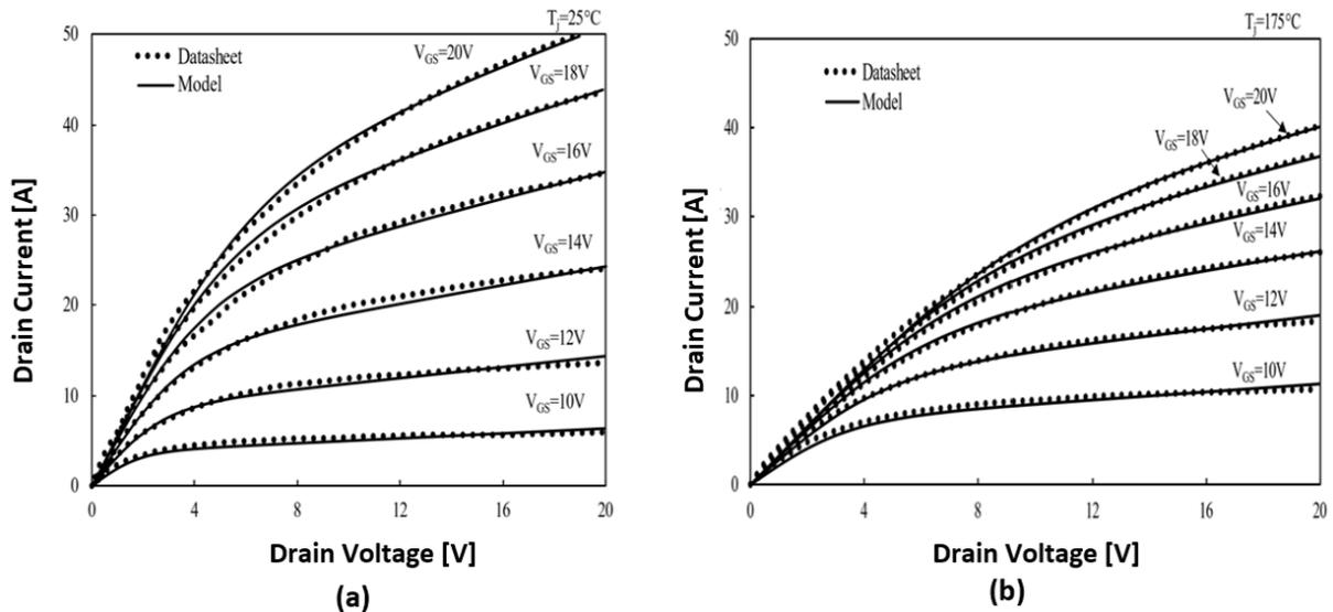
Fig. 4. Output characteristics of the proposed model and CoolSiC MOSFET IMZ120R140M1H from [24] at: a) 25 °C; b) 175 °C.
