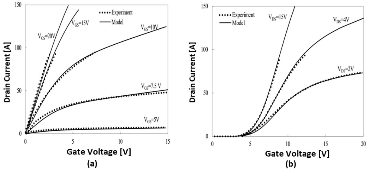
Fig. 7. Static I-V characteristics of model and experimental data obtained from [25]: a) output characteristics; b) transfer characteristics.
