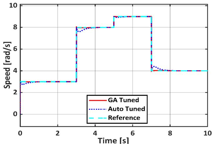
Fig. 15. The controlled transfer function response.
