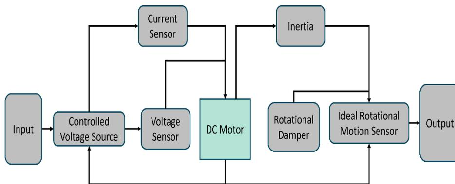
Fig. 4. Block diagram of the SIMSCAPE model.
