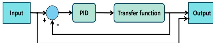
Fig. 12. Block diagram of the system with the PID controller.
