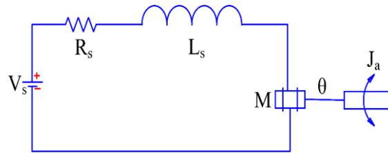
Fig. 2. Circuit diagram of a PMDC motor [31].
