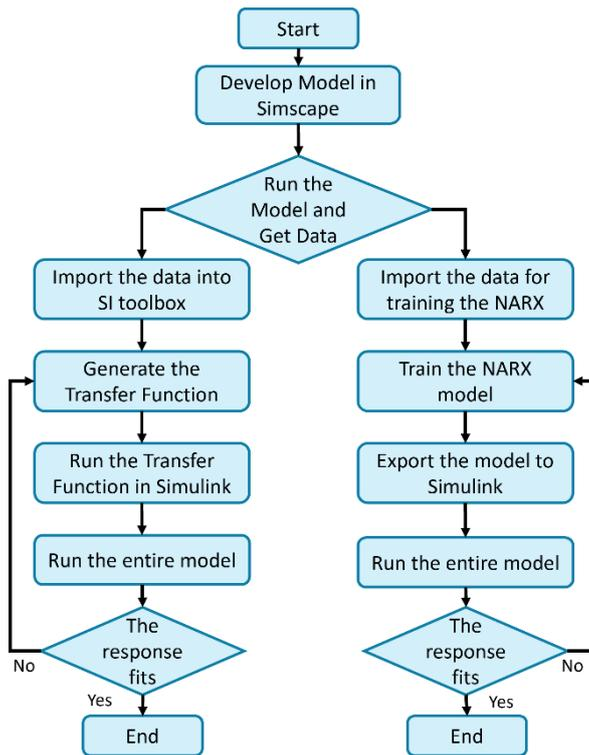
Fig. 3. Flow chart of the transfer function generation and the NARX model training.
