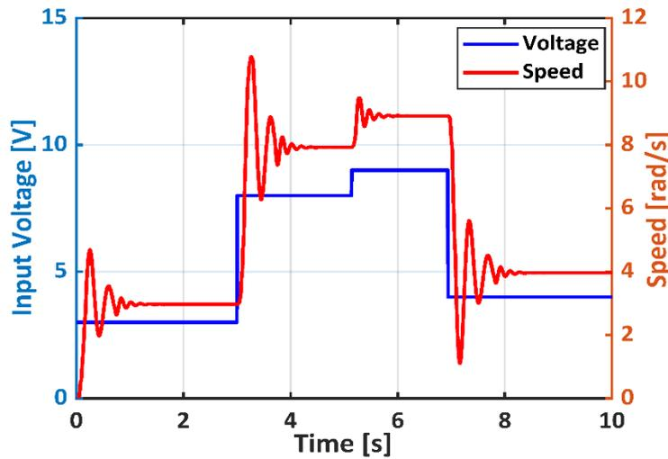
Fig. 8. Response of input voltage and output speed.
