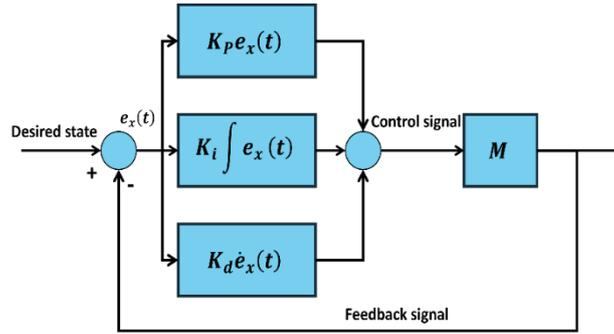
Fig. 7. Schematic diagram of a PID controller [17].
