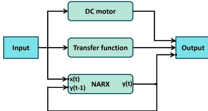
Fig. 9. Blocks of the imported NARX model, transfer function, and DC motor Simscape model for the response comparison.
