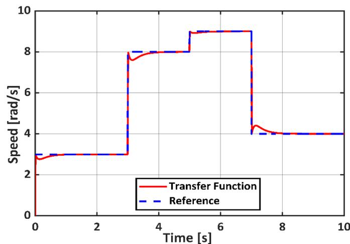
Fig. 13. Response of the system when PID is auto-tuned.
