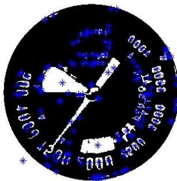
Fig. 4. The centre of the connected area is in the Black-White frame of the dial instrument.
