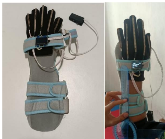
Fig. 5. Hardware implementation of arm and finger movement physiotherapy tools.
