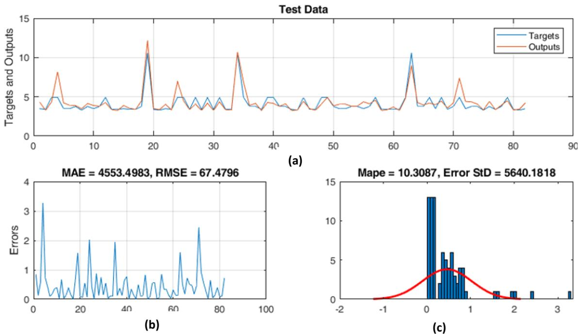
Fig. 5. The results of GMDH-DNN testing on PMSM data to detect the stator winding rings of the SCF: a) random sample number testing data and actual value; b) error among output and actual value; c) the standard deviation error value histogram.
