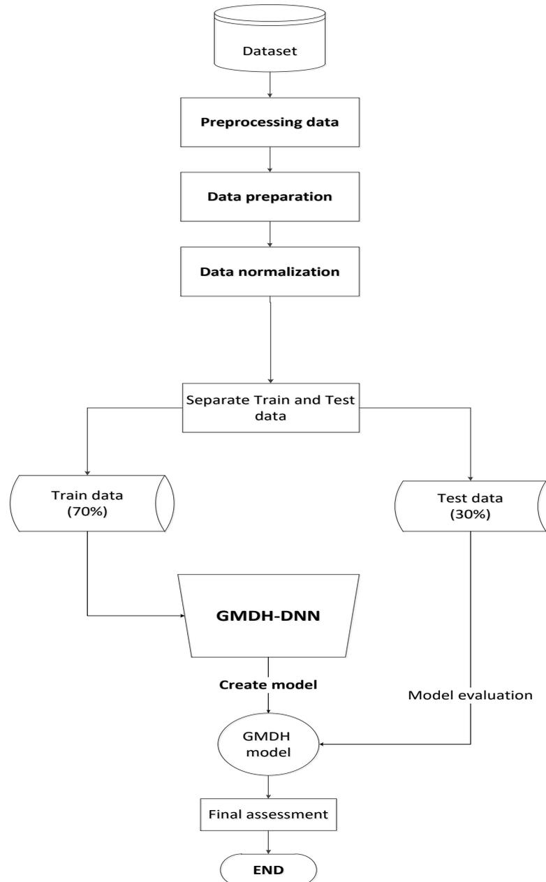
Fig. 1. Architecture of the proposed method for SCF detection in PMSM based-on GMDH-DNN.
