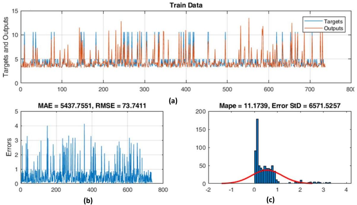
Fig. 4. The results of GMDH-DNN training on PMSM data to detect the stator winding rings of the SCF: a) random sample number training data and actual value; b) error among output and actual value; c) the standard deviation error value histogram.
