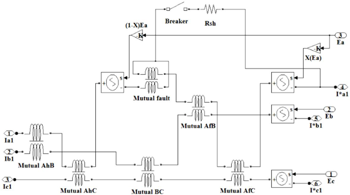
Fig. 2. Circuit model designed for PMSM under SCF condition of in the stator winding.
