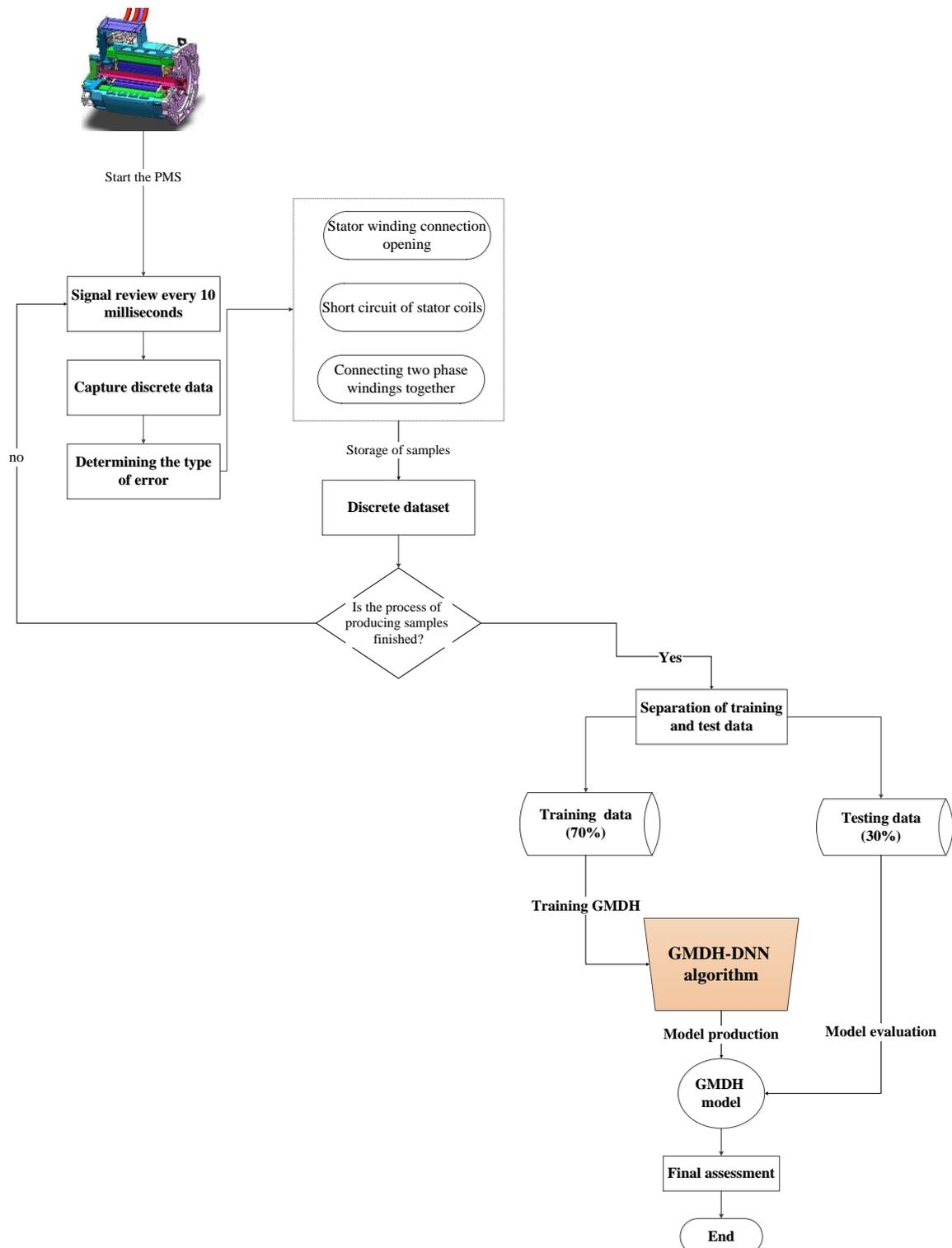
Fig. 3. SCF detection model in PMSM by GMDH-DNN.
