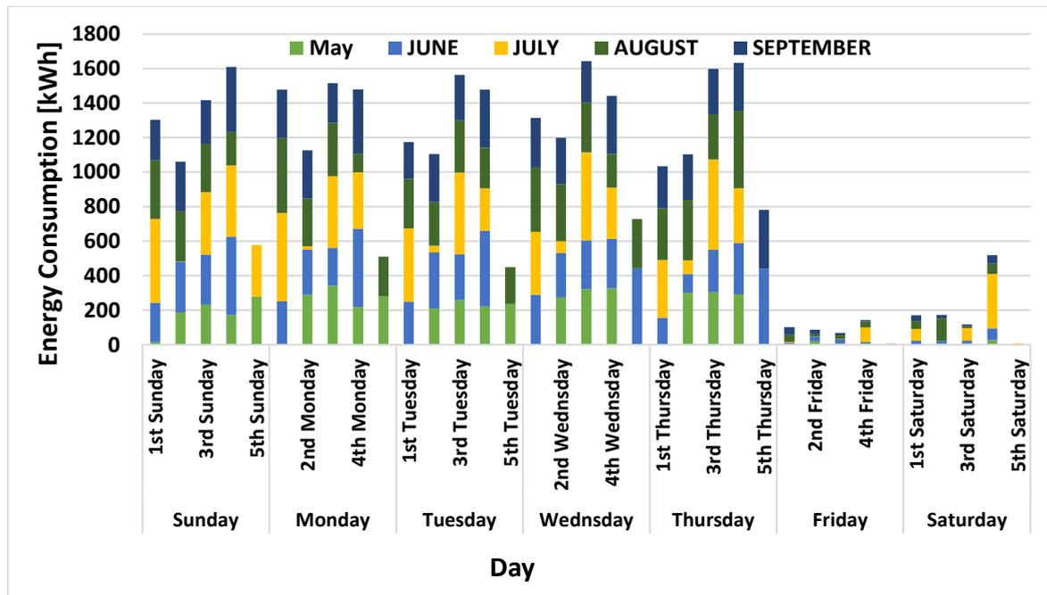
Fig. 13. Daily Consumption of the laboratory building for the period of 5 months in 2022.
