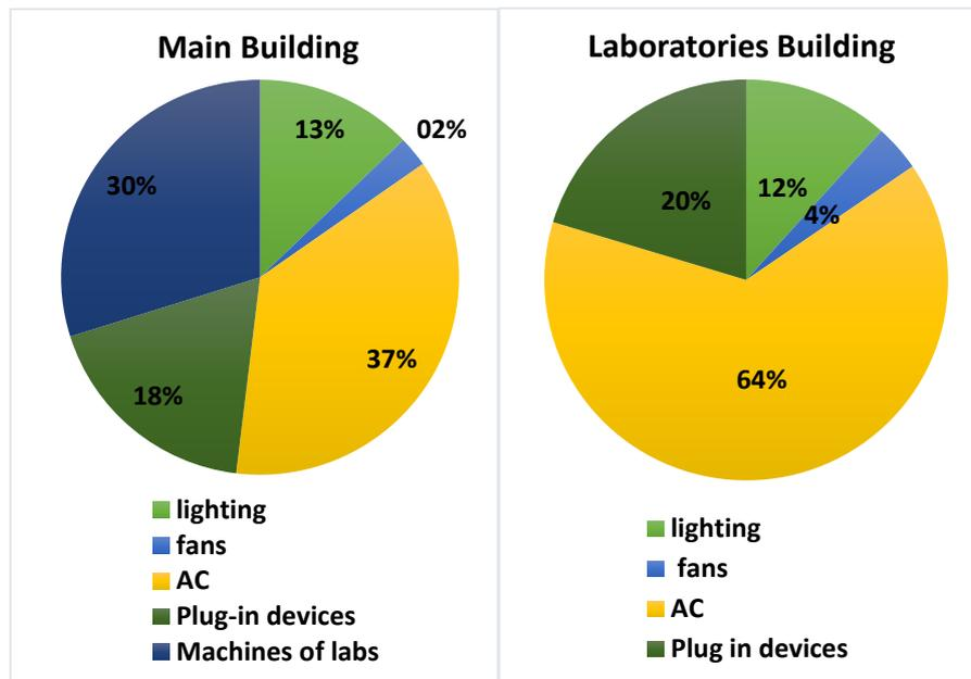
Fig. 10. Percent of load types in the two buildings.
