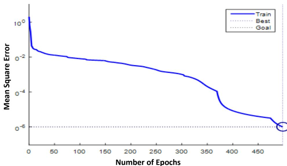
Fig. 11. Performance plot of training the Elman back propagation network.
