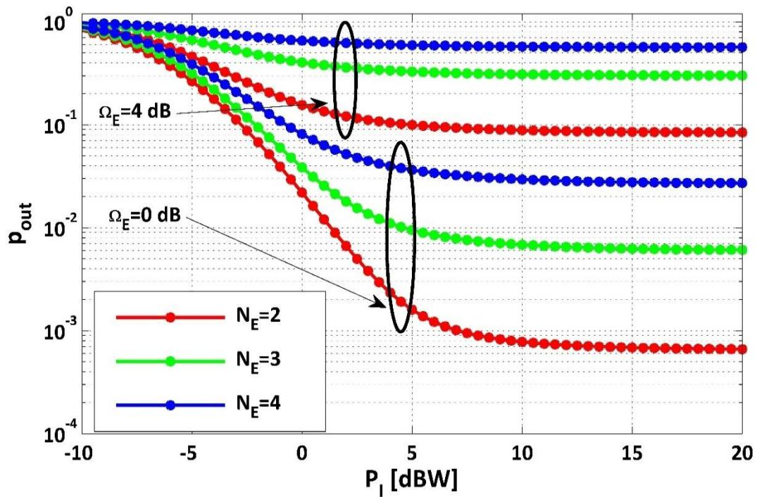
Fig. 5. SOP versus  $P_I$  with  $R_S = R_d = 0.1$ ,  $\beta = \frac{1}{3}$ ,  $\Omega_D = \Omega_p = \Omega_S = \Omega_R = \Omega_t = \Omega_A = 5 \text{ dB}$ ,  $N_D = 3$ ,  $N_R = 2$ ,  $P_t = 10 \text{ dBW}$  and  $m = 2$ .
