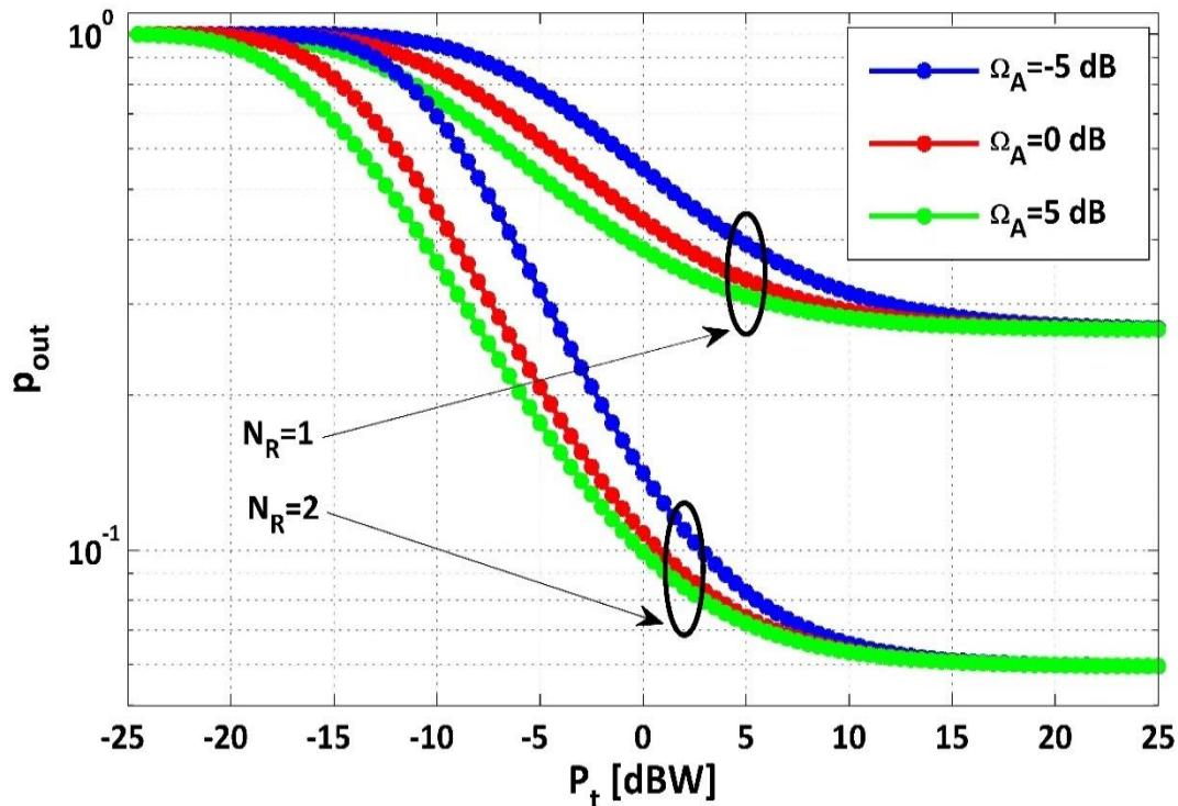
Fig. 4. SOP versus  $P_t$  with  $R_S = R_d = 0.1$ ,  $\beta = \frac{1}{3}$ ,  $\Omega_E = 1$  dB,  $\Omega_D = \Omega_p = \Omega_S = \Omega_R = \Omega_t = 5$  dB,  $N_D = N_E = 3$ ,  $m = 1$  and  $P_l = 10$  dBW.
