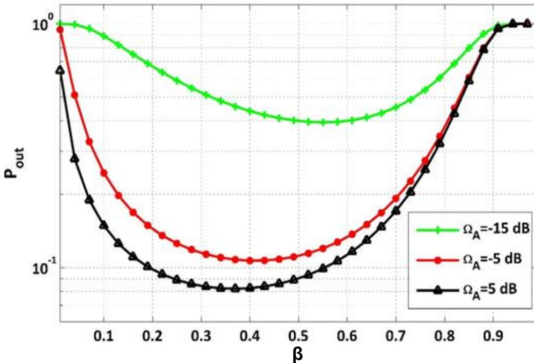
Fig. 8. SOP versus  $\beta$  with  $R_S = R_d = 0.1$ ,  $\Omega_E = 1$  dB,  $\Omega_D = \Omega_p = \Omega_S = \Omega_R = \Omega_t = 5$  dB,  $N_R = 2$ ,  $N_D = N_E = 4$ ,  $P_t = 0$  dBW,  $P_I = 10$  dBW and  $m = 1$ .
