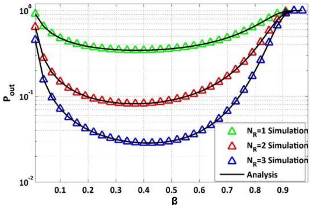
Fig. 6. SOP versus  $\beta$  with  $R_S = R_d = 0.1$ ,  $\Omega_E = 1 \text{ dB}$ ,  $\Omega_D = \Omega_p = \Omega_S = \Omega_R = \Omega_t = \Omega_A = 5 \text{ dB}$ ,  $N_D = N_E = 4$ ,  $P_t = 0 \text{ dBW}$ ,  $P_I = 10 \text{ dBW}$  and  $m = 1$ .
