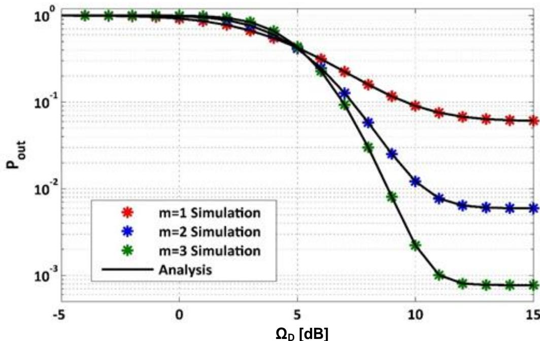
Fig. 2. SOP versus  $\Omega_D$  with  $R_S = R_d = 0.1$ ,  $\beta = \frac{1}{3}$ ,  $\Omega_E = 1$  dB,  $\Omega_p = \Omega_S = \Omega_R = \Omega_t = \Omega_A = 5$  dB,  $N_E = 4$ ,  $N_D = N_R = 2$ ,  $P_t = 1$  W and  $P_I = 2$  W.
