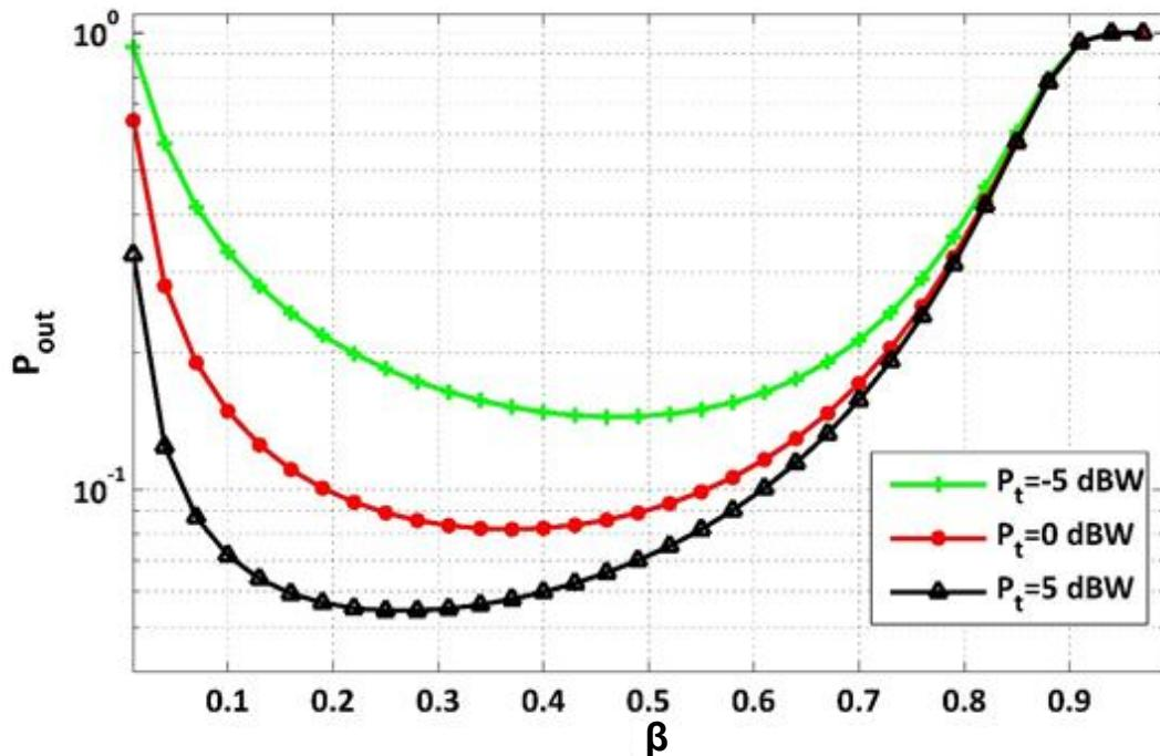
Fig. 7. SOP versus  $\beta$  with  $R_S = R_d = 0.1$ ,  $\Omega_E = 1$  dB,  $\Omega_D = \Omega_p = \Omega_S = \Omega_R = \Omega_t = \Omega_A = 5$  dB,  $N_D = N_E = 4$ ,  $N_R = 2$ ,  $P_I = 10$  dBW and  $m = 1$ .
