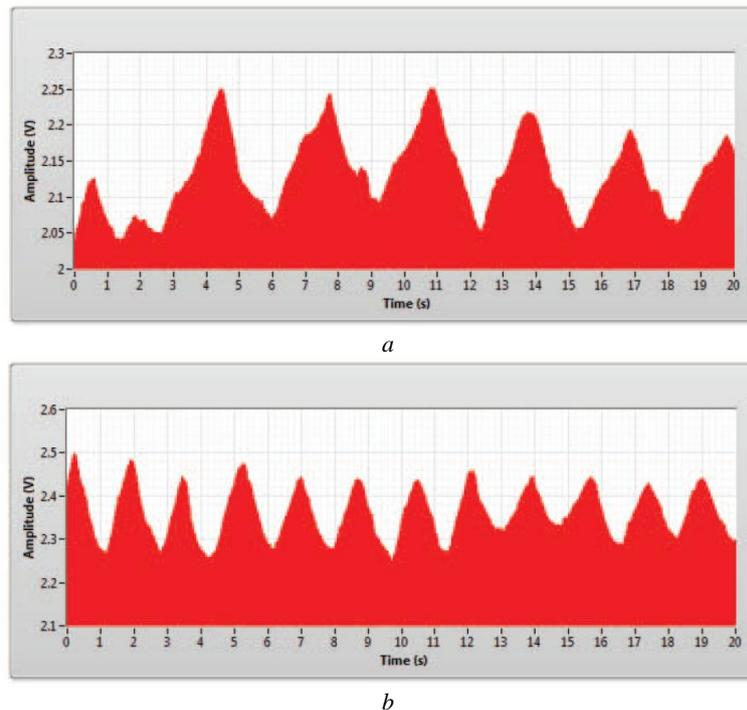
Fig. 11. a) A 20-second deep breathing rhythm on top of the underwear, b) A 20-second increased breathing rhythm on top of the underwear
