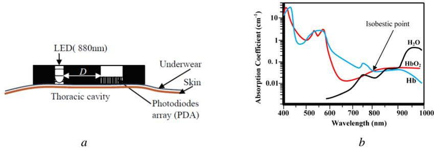
Fig. 2. a) Cross section view of the respiration rate sensor placed on the thoracic cavity, b) Optical window
