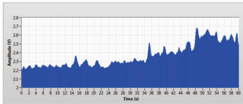
Fig. 14. Chaotic breathing measured on top of the underwear
