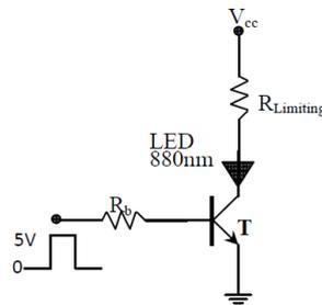
Fig. 3. NIR LED driver circuit
