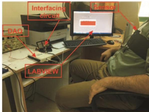
Fig. 4. An image for the system used in the measurements
