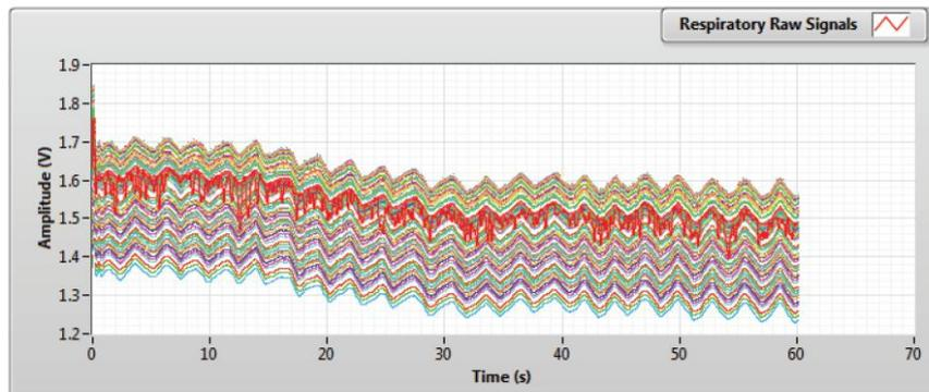
Fig. 6. The de-multiplexed signals as generated by 128 photodiode arrays
