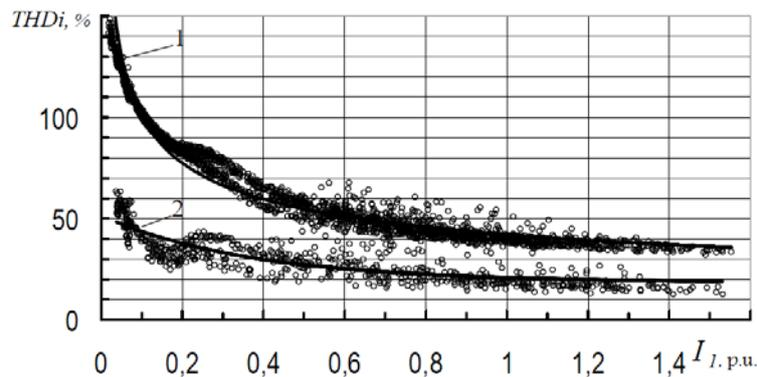
Fig. 7.  $THDi = f(I_l)$  curves for inverter type Altivar 71, 5.5kW. 1- with the current filter recommended by the manufacturer (Schneider Electric Co.), 2- with the current filter suppressing the 5<sup>th</sup>, 7<sup>th</sup> and 11<sup>th</sup> harmonics
