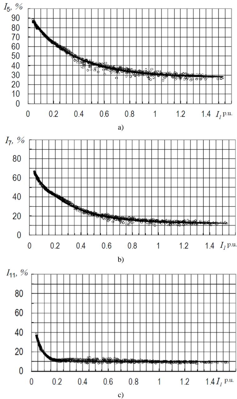
Fig. 5. Spectral analysis of line current waveforms in Fig. 4 are shown for the 5<sup>th</sup>, 7<sup>th</sup> and 11<sup>th</sup> harmonics as a function of the load on the inverter
