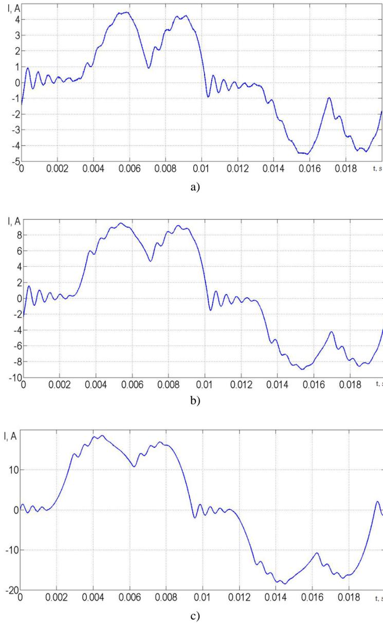
Fig. 4. The line current waveforms of inverter type Altivar 71 (5.5kW) when the inverter was a) 25% loaded, b) 50% loaded and c) 100% loaded
