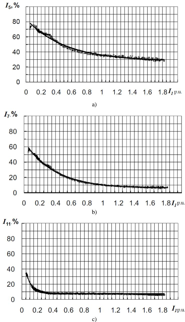
Fig. 3. Spectral analysis of line current waveforms in Fig. 2 are shown for the 5<sup>th</sup>, 7<sup>th</sup> and 11<sup>th</sup> harmonics as a function of the load on the inverter
