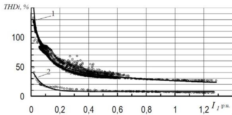
Fig. 6.  $THDi = f(I_1)$  curves for inverter type Altivar 71, 2.2kW. 1- with the current filter recommended by the manufacturer (Schneider Electric Co.), 2- with the current filter suppressing the 5<sup>th</sup>, 7<sup>th</sup> and 11<sup>th</sup> harmonics
